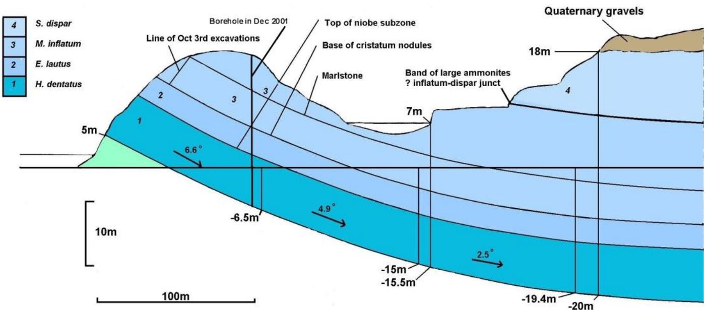
Dip values are calculated and based on the height of the Gault base at intervals of 100m NE of the boundary of the main lake. Thicknesses are based on the log, calculated from the base of the Gault (5m OD), the north side of the upper lake (7m OD) and the junction with the Quaternary gravels (18m OD).
