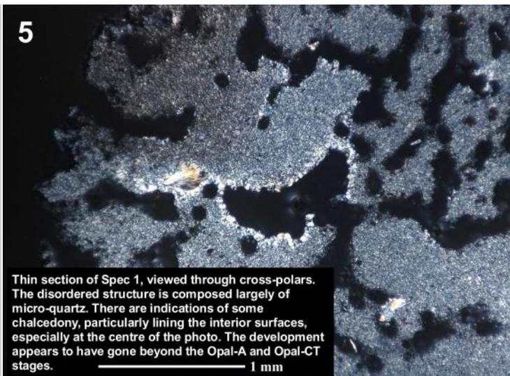
Thin section of Spec 1, viewed through cross-polars. The disordered structure is composed largely of micro-quartz. There are indications of some chalcedony, particularly lining the interior surfaces, especially at the centre of the photo. The development appears to have gone beyond the Opal-A and Opal-CT stages.
